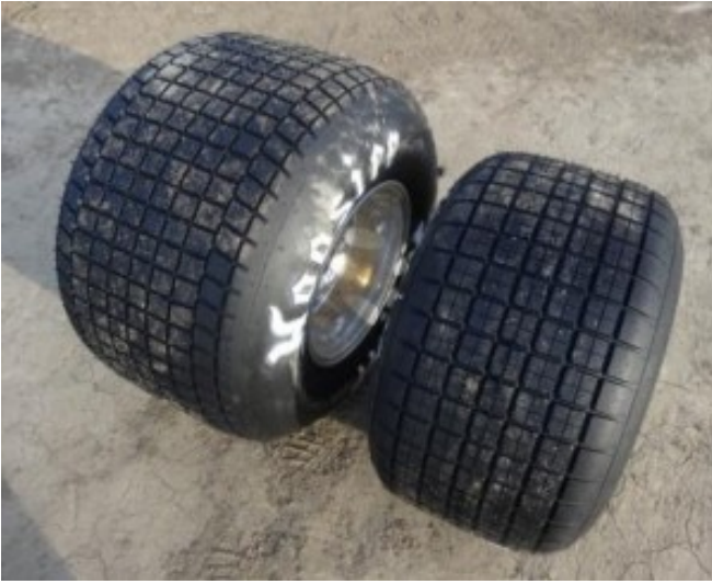
2016 SOD spec tires. 100/13-15 medium and 92/12.5-15 D15
