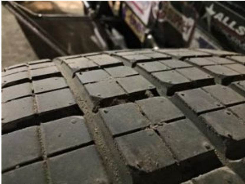
Left rear after a full night and 25 lap feature on a \frac{1}{2} mile track.
