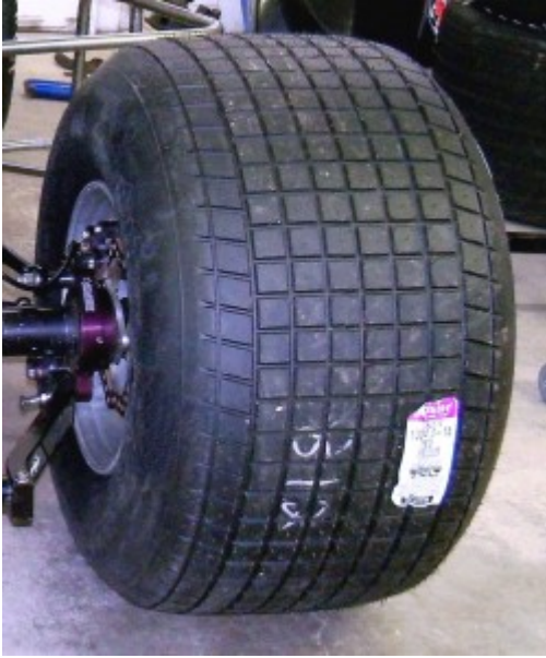
The SOD right rear is a Hoosier 100/13-15, medium compound.
